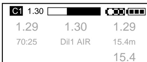
Towards the end of the scrubber activity the software changes the display so the scrubber monitor works more like the fuel gauge on a car. i.e. when the gauge is empty you cannot stay on the rebreather and open circuit bailout should be used.
