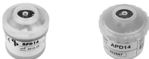
Three galvanic oxygen sensors are fitted to each rebreather. Two types are currently used, APD14 and APD16, each from a different manufacturer. Both feature the SMB co-axial connector, hydrophobic membranes and other common characteristics to allow use in the high humidity and temperature range experienced inside the breathing circuit.
