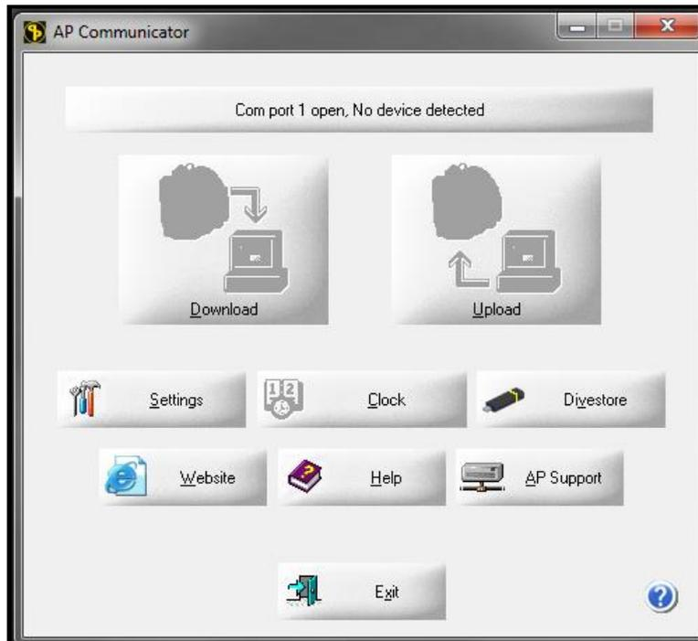
3. Once installed run the AP Communicator, select Settings and choose the COM Port. If the COM Port No. is unknown this can be checked using the PC's Device Manager in Control Panel. The available ports are shown on the Settings screen.
