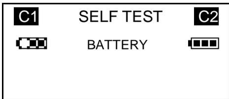
The batteries are tested while the solenoid fires and battery voltage is reflected in the icons.
