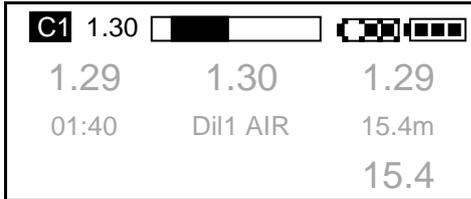
If the scrubber is used for another dive, the bottom of the scrubber rarely heats up, indicated by the clear left hand side of the scrubber monitor.
