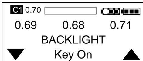
If Key On is selected, the backlight is normally off but comes on when a switch is pressed. The left switch operates the backlight for 5 seconds, the centre or right switch operates the backlight for 15 seconds.
